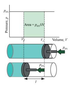
• Work done (W) on an ideal gas in a cylinder when it is compressed by constant pressure,  $p_{ex}$  can be derived as follows:
